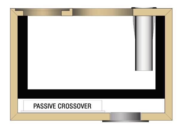
With the passive crossover in place, find the input terminals and feed them out through the rear opening. insert the black acoustic lining, which covers the rear, top and bottom internal faces of the enclosure. Check that it does not block the internal opening of the port. Glue is not necessary.
