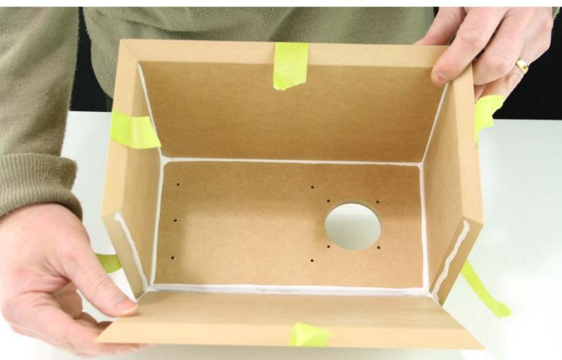
Apply a single thick bead for the top and side panels. Test the first pair of mitres to confirm glue coverage, then glue and fold up all the other panels. It is best to fold up and then tape one join at a time. Ensure the glue covers the join before moving on to the next step.
