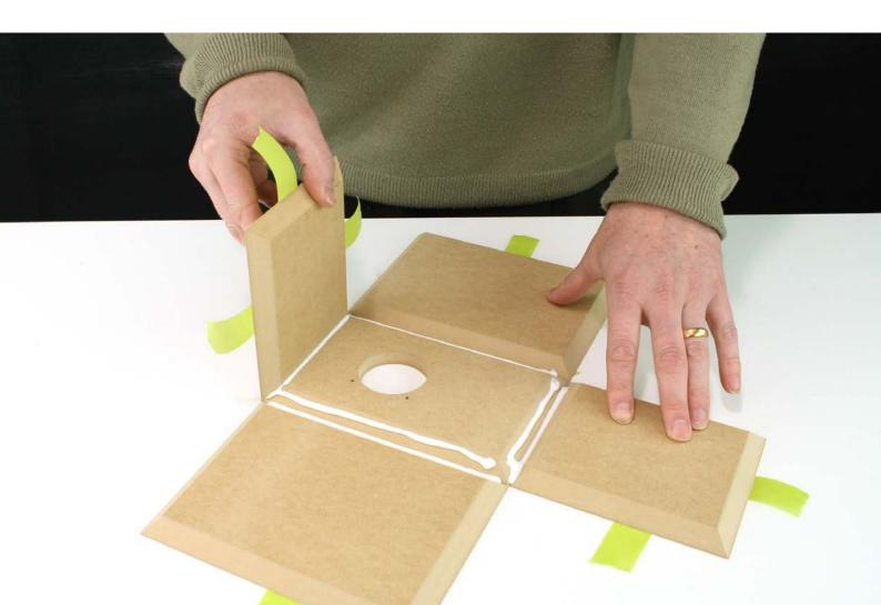
Confirm the amount of glue applied by folding up the first panel. The glue should cover the entire surface in contact. It's preferable to see the glue ooze beyond the join slightly. This provides visual feedback on whether the glue has set. Once set, PVA glue becomes transparent.
