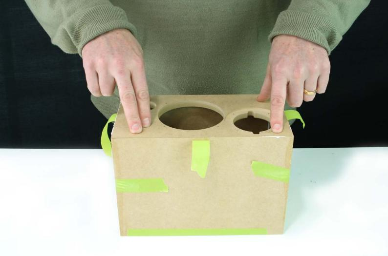
Once you have confirmed adequate glue coverage, press the baffle into place and wipe off all excess glue with a damp cloth. Secure panels firmly with masking tape. Apply pressure when pressing the tape into position. The tape holds the panels together as the glue sets.
