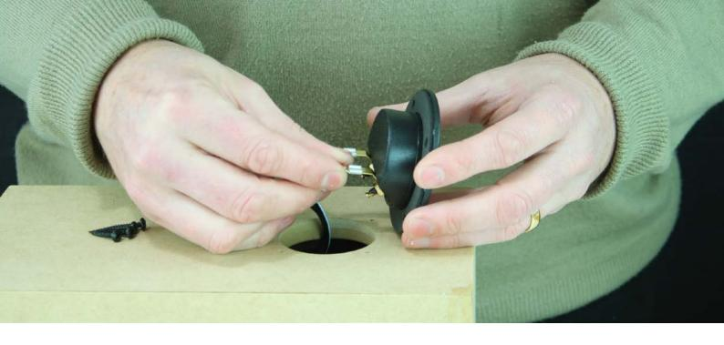
We recommend using a Phillips head screwdriver, as some powered drivers are more likely to cause damage if the head slips off the screw head. Impact drivers should be avoided. If using a powered driver, it's best to use one which has a clutch, so that once the screws are adequately tightened, the driver will not over-tighten. This avoids stripping the MDF pre drilled holes or damage to the screw heads. If using a screwdriver, your left hand can hold the shaft to avoid slipping.
