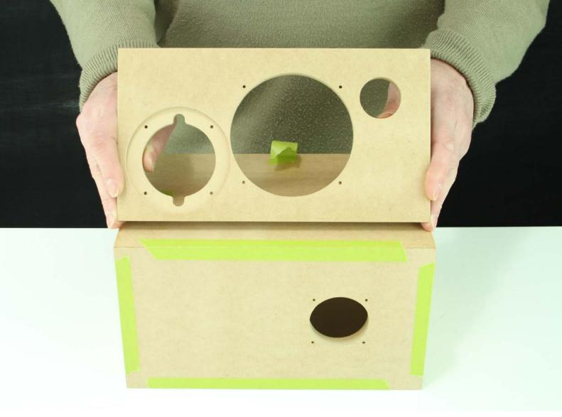
Ensure the front baffle has the correct orientation. The port on the front and terminals on the back should be oriented so they are both on the bottom. In the picture above they are both on the right as the speaker is placed on its side.
