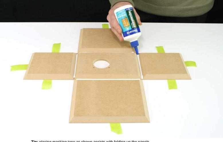
**Tip:** placing masking tape as shown assists with folding up the panels.
